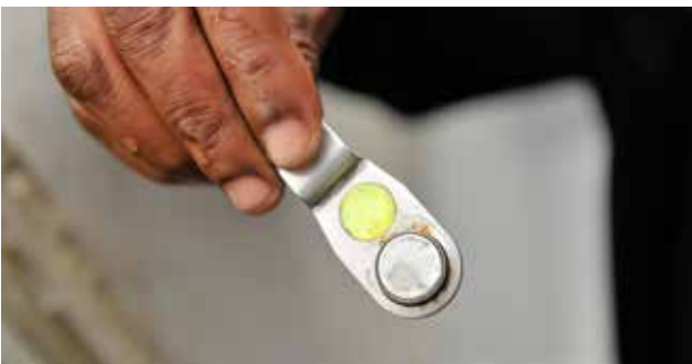
Innovative technology makes it possible for a backyard tenant to swipe a tag to discharge a free monthly supply of water. When the free limit is used, the trickle system kicks in or additional units can be bought.
