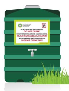
**'Do not drink' warning signs must be placed** at the property's main thoroughfare (i.e. at the entrance gate) and the point(s) of use, and all pipes that are used in the alternative water system also need to be colour-coded. (See the full guideline documents for the colours required.)
