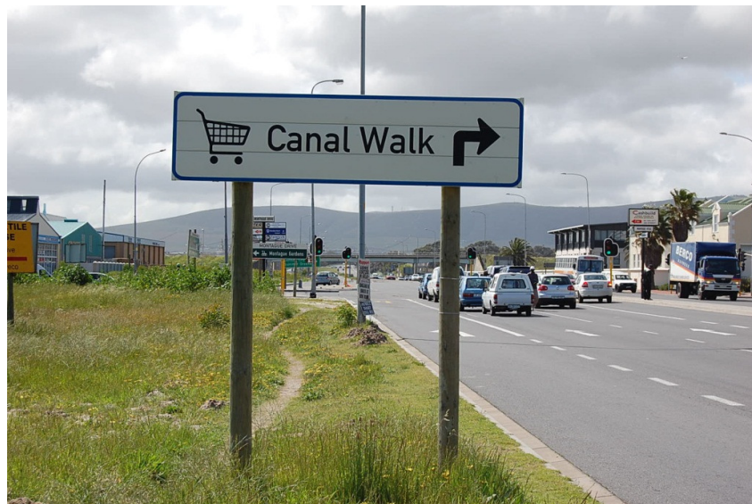
Fig 5. Example of a Guidance Local Sign normally displayed only once the motorist has reached the Suburb of Century City where the facility of Canal Walk is located
