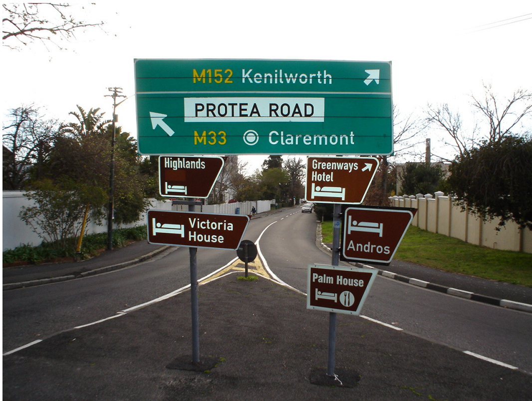
Photograph 3. Illegal Tourism Signage (brown signage) - A classic example of uncontrolled tourism "advertising" and an "overload" of information. All these tourism signs are incorrectly positioned. The primary signage (green sign) is complete in the display of "Primary Information" i.e. Road Name, Route Numbers and Suburb Guidance/Orientation.
