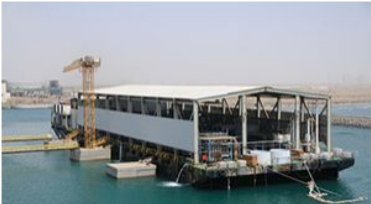
Figure 2 – 50 MLD Barge-based SWRO Desalination Plant in Yanbu, Saudi Arabia
