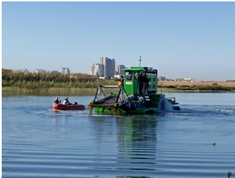
Figure 2: The new weed harvester, the Otter, in Table Bay Nature Reserve.
