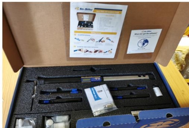
Figure 107: Bought with capital funds, the Aquatroll600 is a specialised water monitoring device which provides water quality parameters in real time. This will greatly help when responding to sewage spills, blue green algae blooms and salinity levels.
