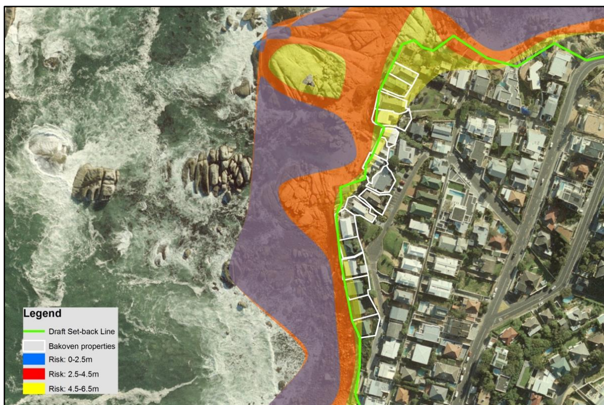
Figure 4: Private property in Bakoven at risk from storm surges
