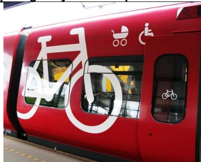
Figure 26: Seating in the middle of the S-train is less popular with passengers and is therefore used as bicycle compartments. 7
