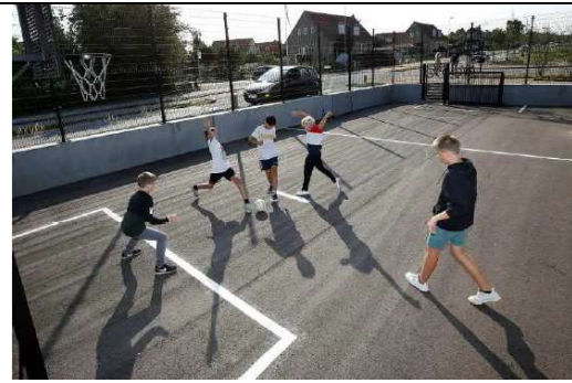
Figure 38: Sunken recreational areas that double up as retention ponds during heavy rain episodes to prevent flooding.
