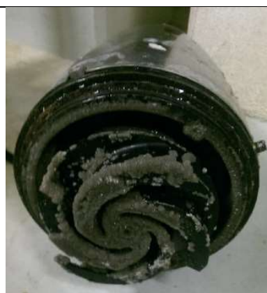
Figure 34: Scaling in WWTP pumps
