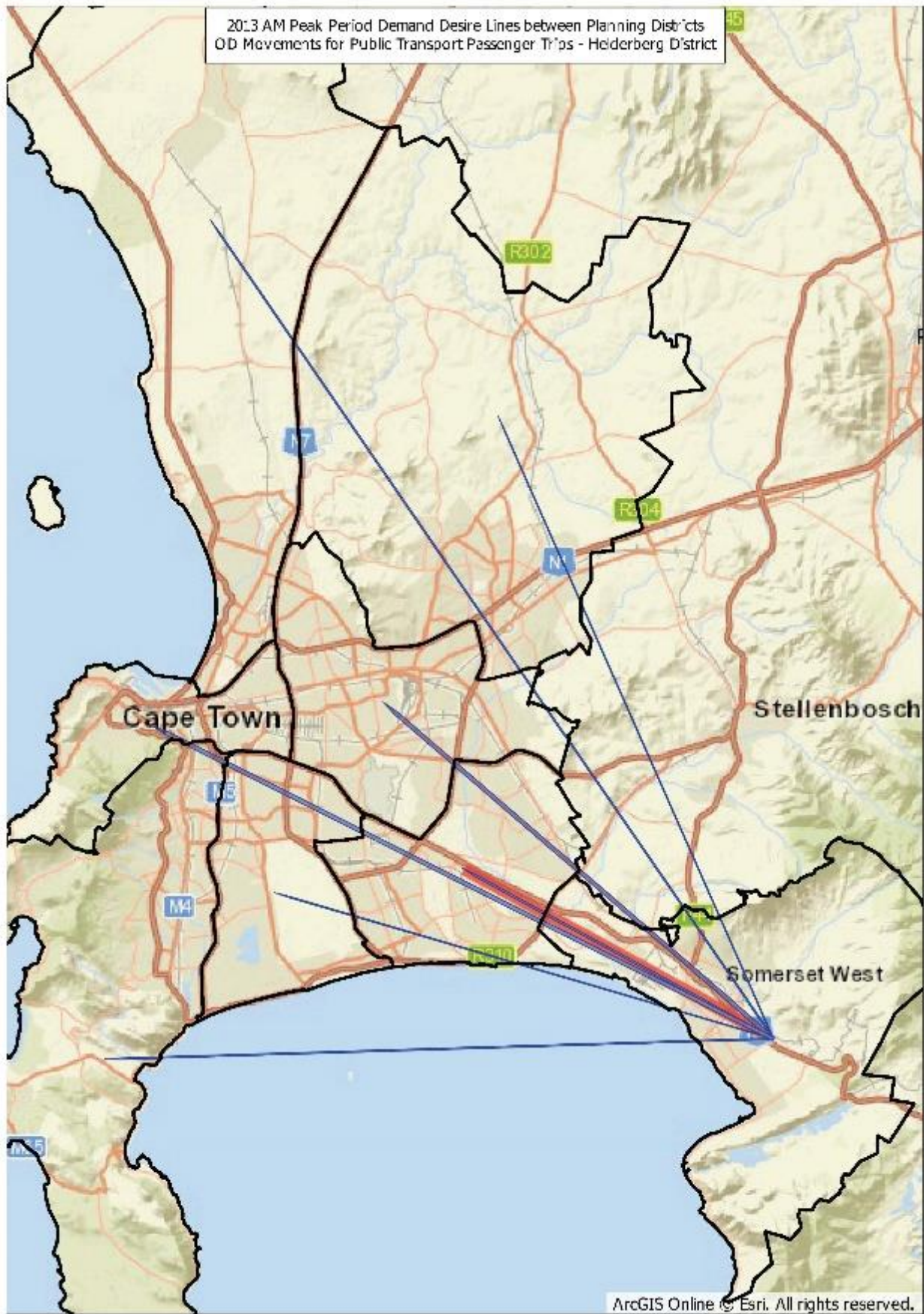
Figure 34: Origin-destination mapping of peak morning commuter trips by public transport in relation to the Helderberg District, 2013 (EMME Travel Demand Modelling, 2013)
