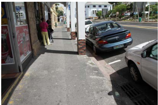
13. Pedestrian crossing makes no provision for the blind. Textured pavers and traffic lights that produce a sound when it is safe to cross should be introduced
