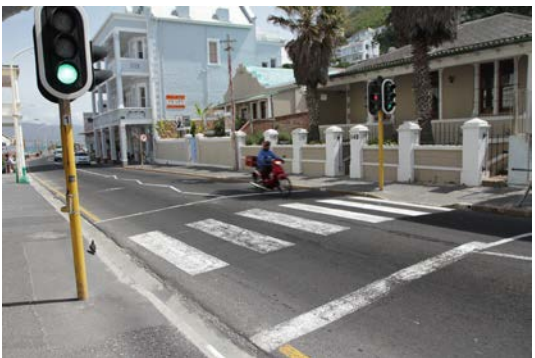
13. Pedestrian crossing makes no provision for the blind. Textured pavers and traffic lights that produce a sound when it is safe to cross should be introduced
