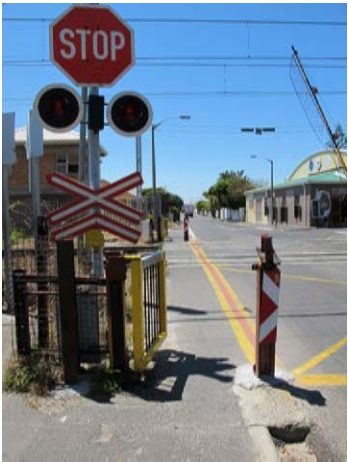
19. A pedestrian gate on one side indicates which side of the route to walk but a change in surface would be more legible to pedestrians
