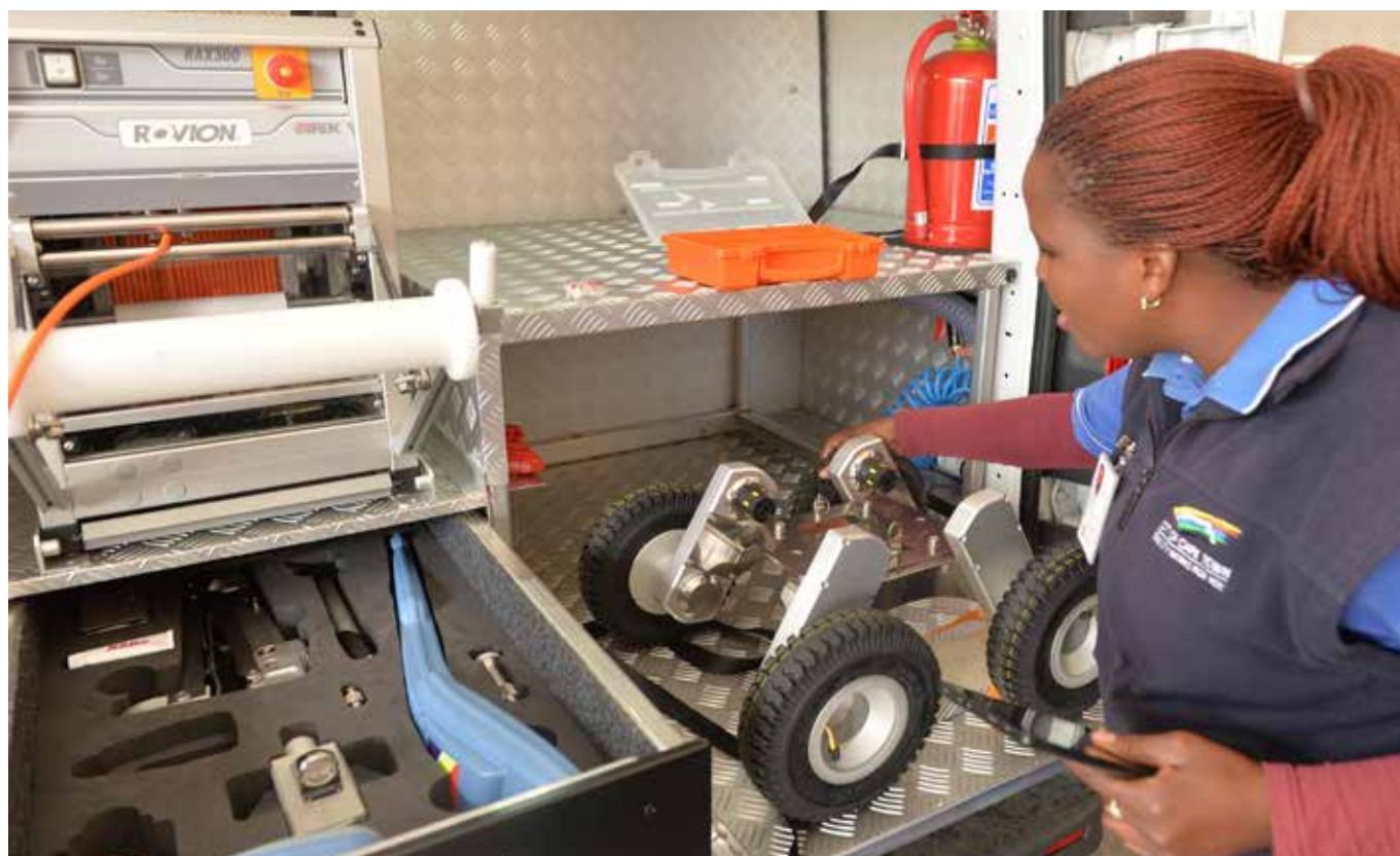
The new closed-circuit television pipe inspection technology – the robotic crawler – was introduced to help monitor the City's water and sanitation infrastructure.
