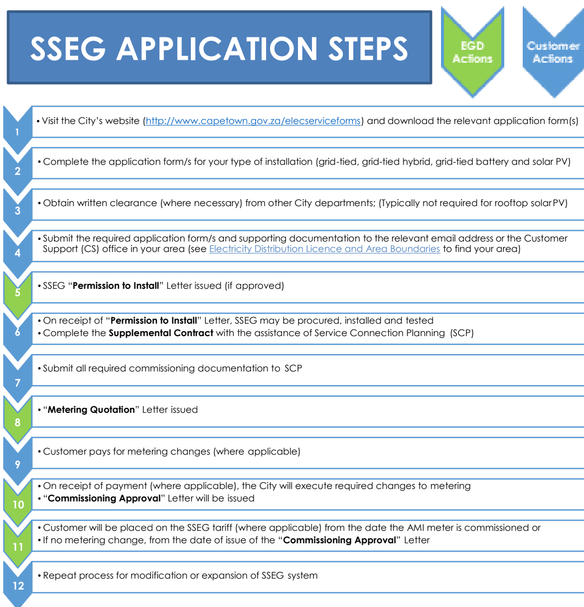
Figure 1: SSEG Application and Approval Process
