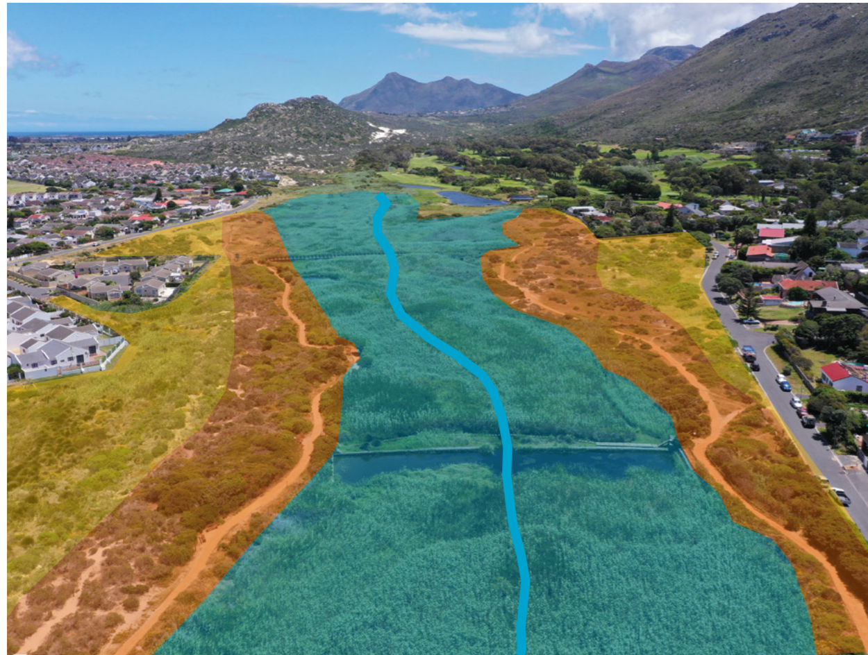
Figure 20: Silvermine River wetlands showing the buffer zone on either side, which includes for appropriate recreational infrastructure, maintenance access, and helps protect the watercourse and wetland from impacts of urbanisation. Blue line – river channel (notional); green overlay – wetland; dark orange overlay – buffer; lighter orange overlay – buffering open space.
