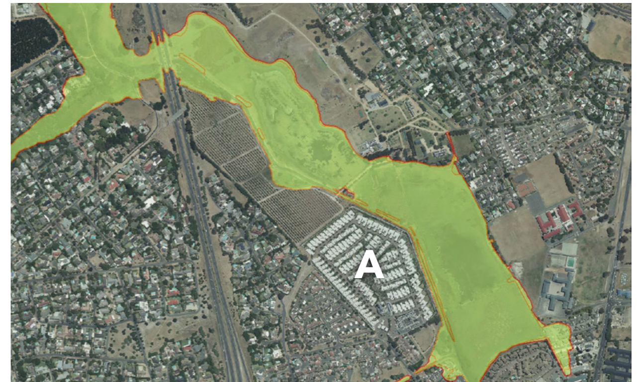
Figure 6: Aerial photograph with 1:50-year (orange) and 1:100-year (red) floodlines and floodplain (green) superimposed on it. Note the recent development (A) is located outside of them.
