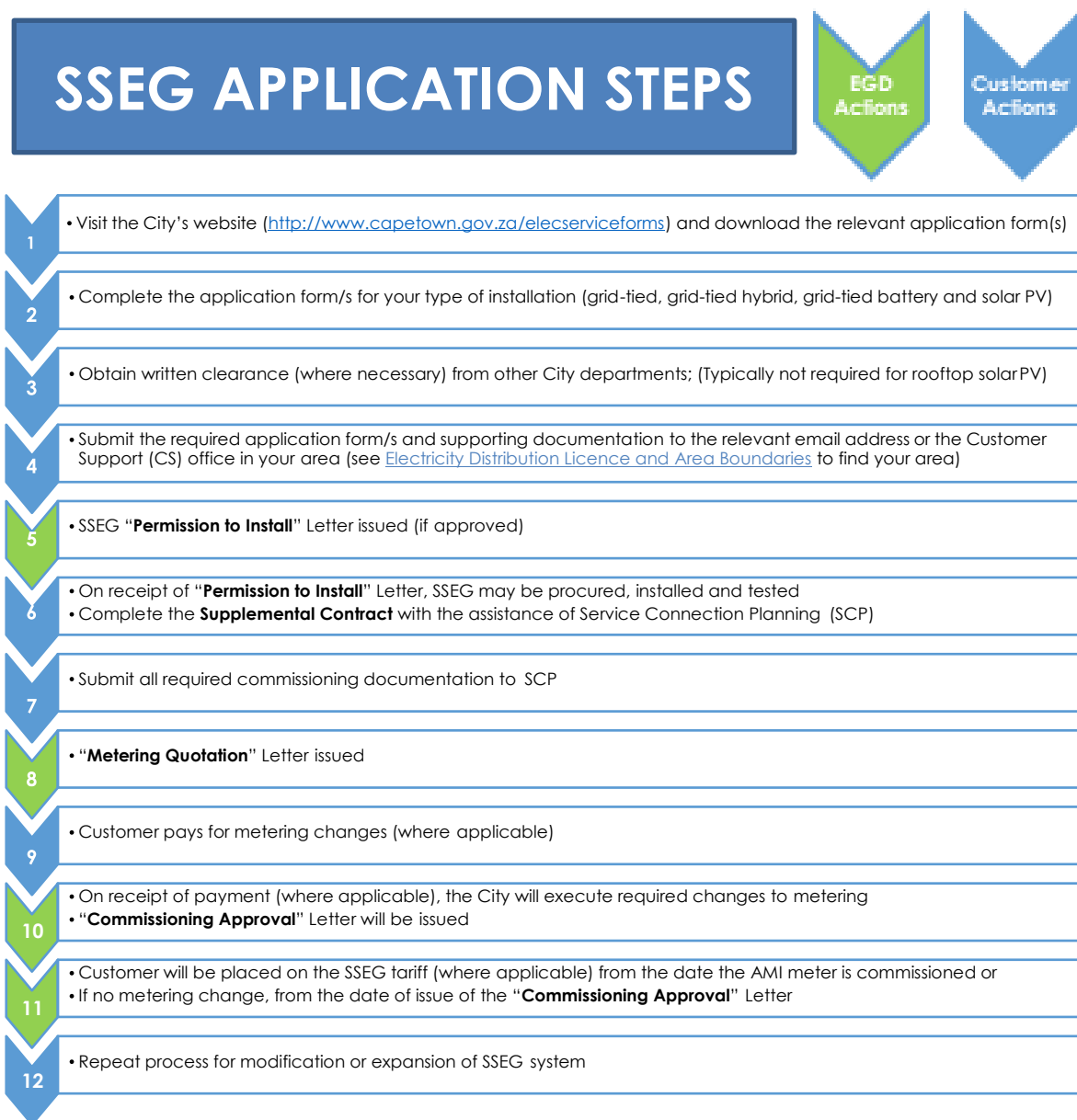
Figure 1: SSEG Application and Approval Process
