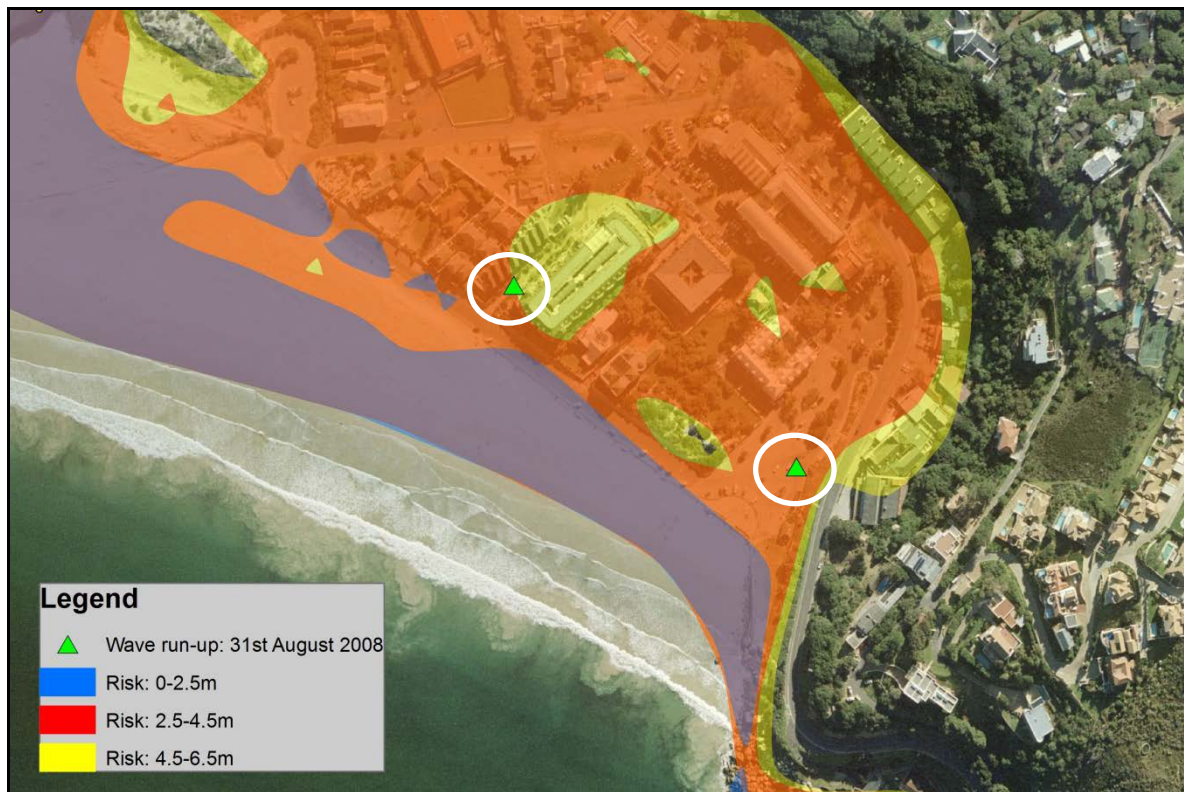
Figure 4: Wave run-up measurements taken from an actual storm event with a differential GPS and overlaid with the GIS inundation model
